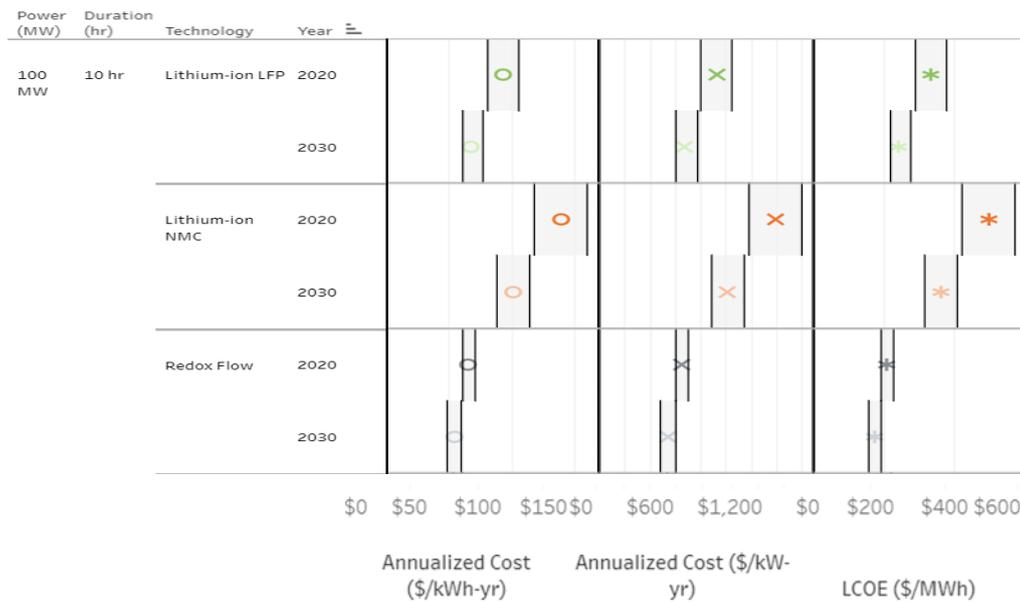
**Fig. 12 Utility-scale stationary battery cost outlook (2020 and 2030)**
