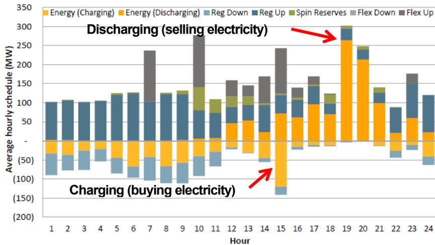
**Fig. 3 Average real-time battery schedules in California (September 5 and 6, 2020)**
