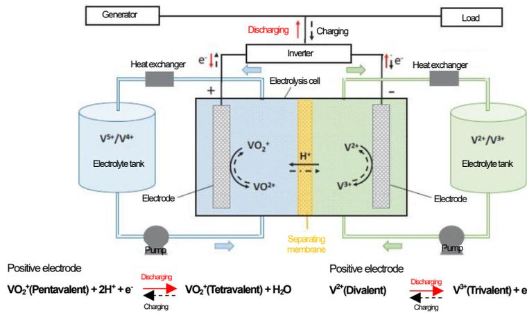
Fig. 4 Operating principle of RFB<sup>6</sup>
