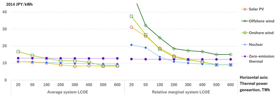
Fig. 5 Calculation of average and marginal System LCOEs
