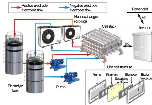
Fig. 5 Cell stack configuration details<sup>7</sup>
