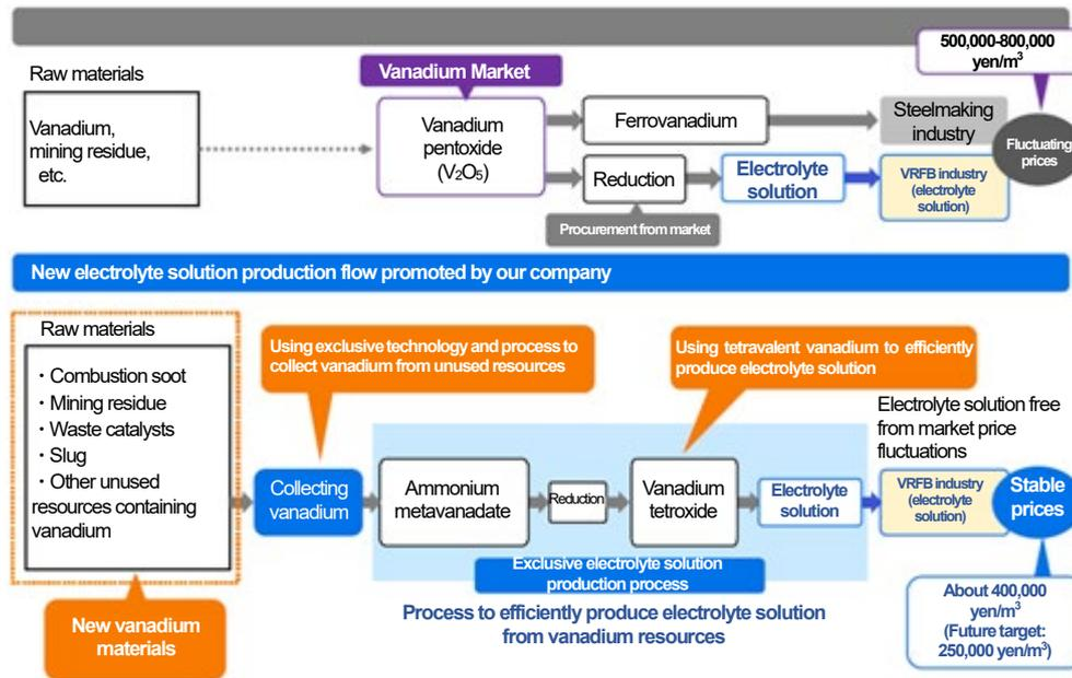
**Fig. 16 Innovative vanadium electrolyte solution production flow**
