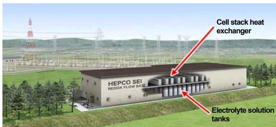
**Fig. 14 Conceptual drawing of a large VRFB system to be introduced by HEPCO**
