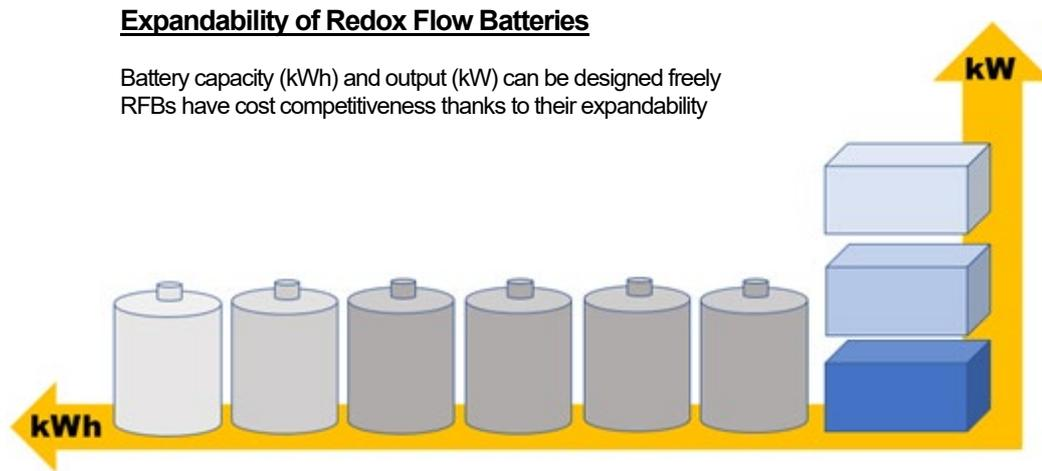
**Fig. 9 Conceptual diagram of RFBs' expandability**
