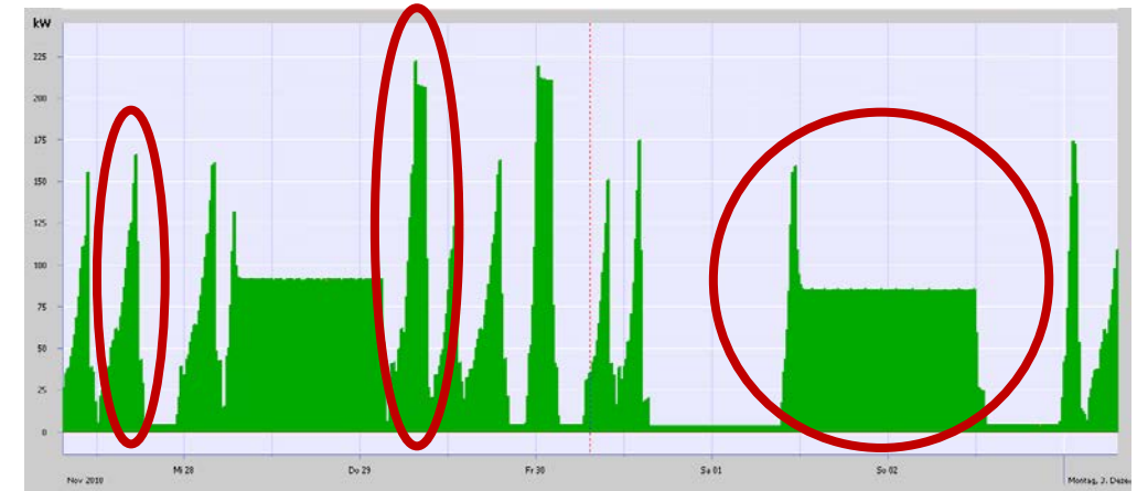
Brazing furnace with 3 typical production related load profiles
