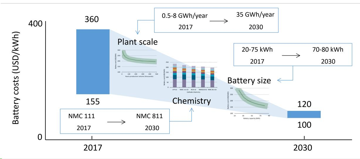
The combined effect of manufacturing scale up, improved chemistry and increased battery size explain how battery cost can decline significantly in the next 10 to 15 years
