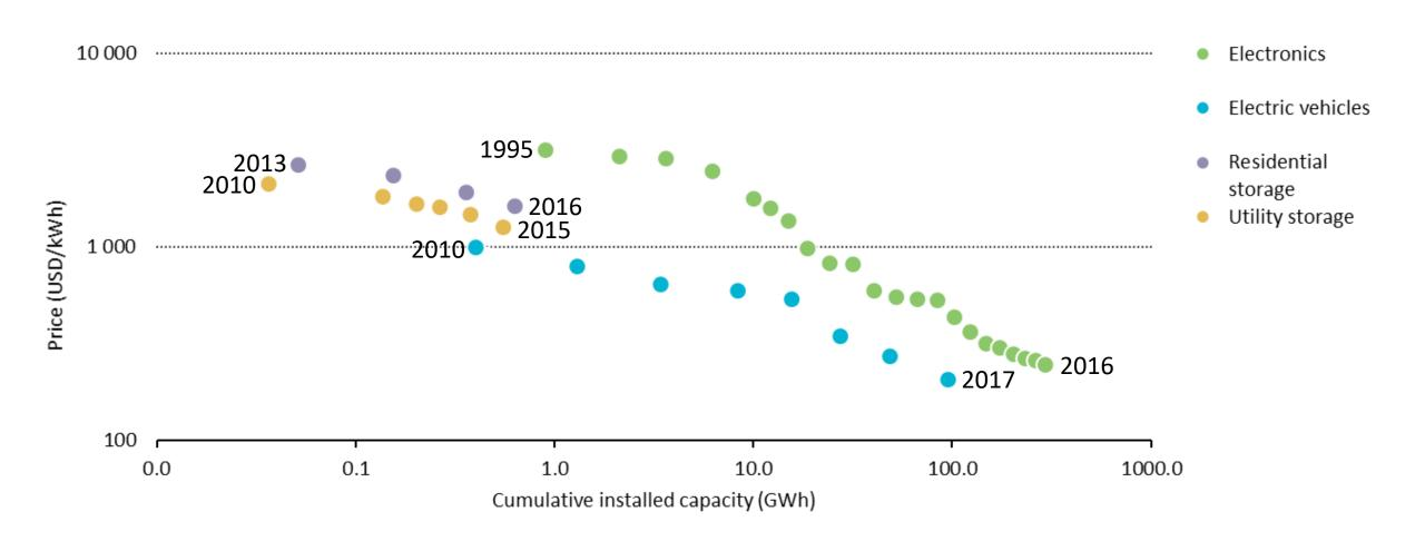
Consumer electronics led to cost declines (through technology progress and scale) for Li-ion in the past This benefited both EV packs, now set to deliver the next scale up, and stationary storage
