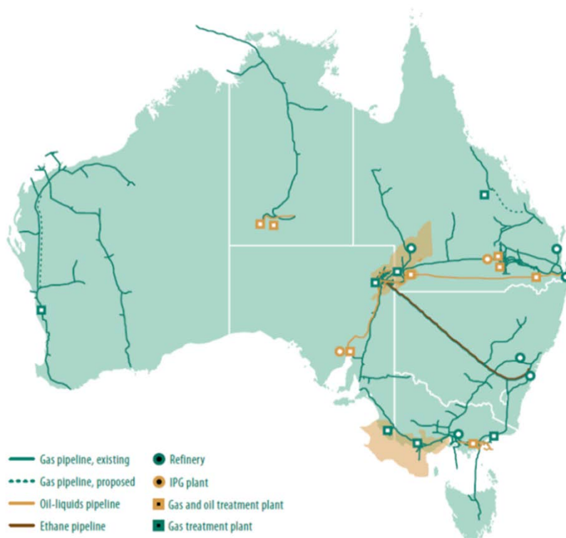
Figure 30 Australia’s natural gas pipeline infrastructure
