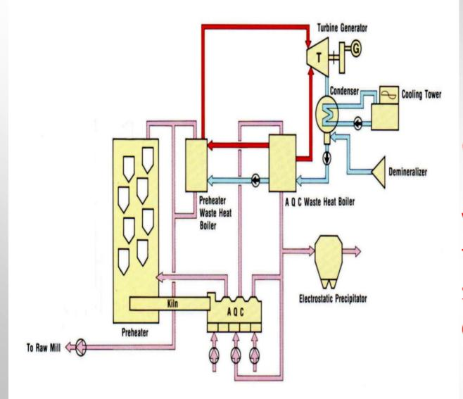
Generating power using waste heat from kiln and supplying it to cement production
