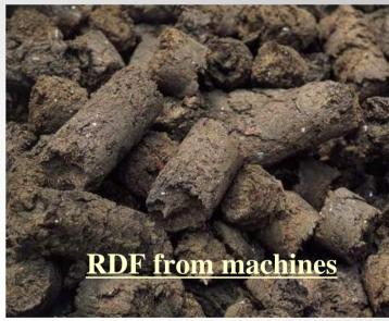
Waste Pachinko machine, will be processed into RDF after crushing and kneading.
