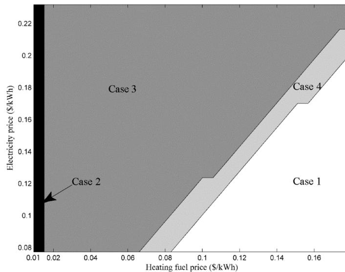
Figure 8 Optimum design case changes as the electricity and heating fuel prices change.
