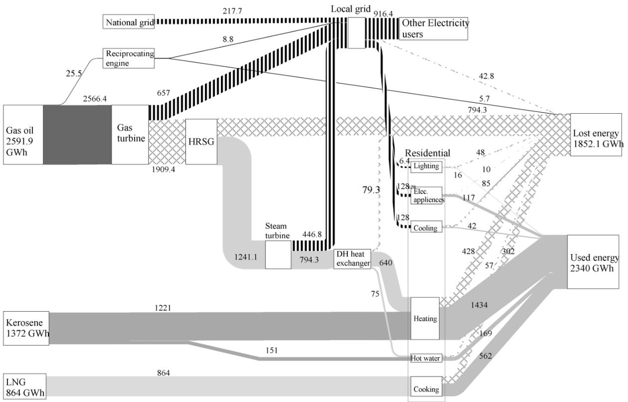
Figure 6 Energy flow for the energy optimum design (Case 3).
