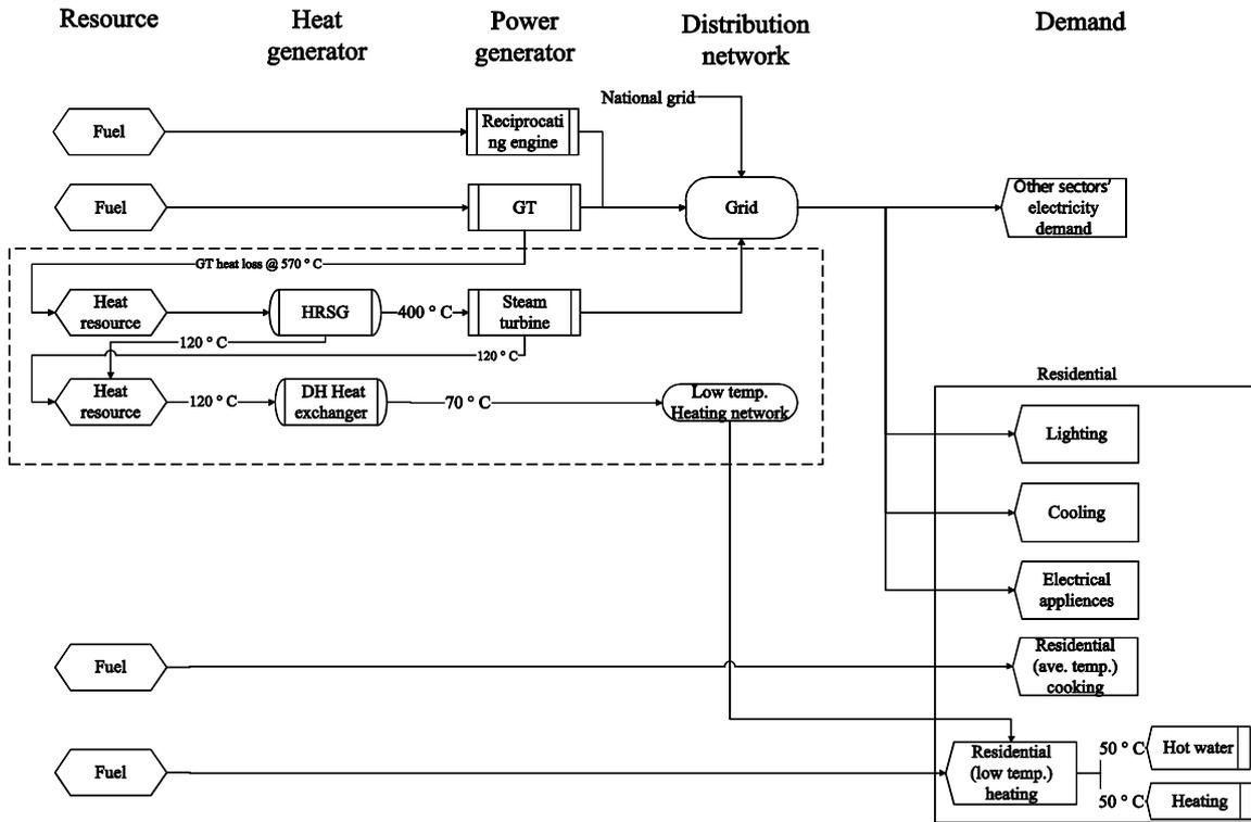
Figure 4 The system diagram of the general configuration of the energy system.
