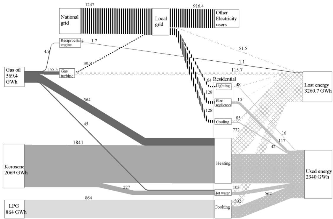
Figure 2 The energy flow diagram showing the quantitative flow of energy at the time of data collection in the analyzed system.
