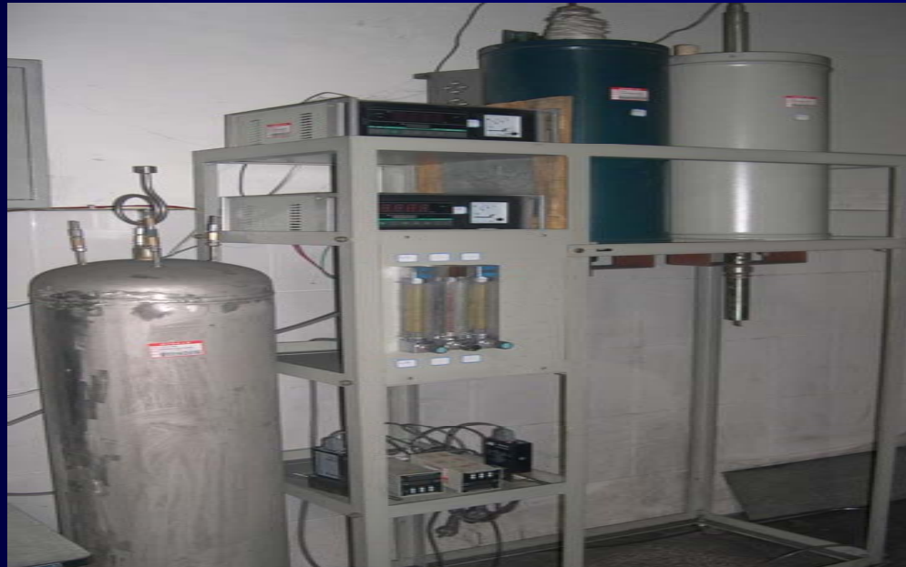
Fig.9 Atmospheric carbon - calcination cycle of test-bed
