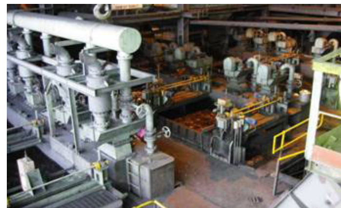
Jig Washers after Modification
