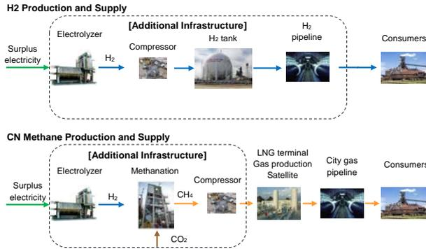
**Figure 11** Facility configuration for hydrogen supply and CN methane supply
