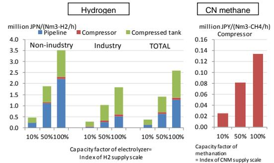
**Figure 12** Unit cost of supply infrastructure for hydrogen and CN methane
