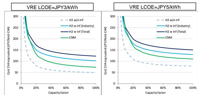
**Figure 14** Comparison of supply costs for hydrogen and CN methane
