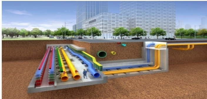
Figure-18 Piping arrangement
